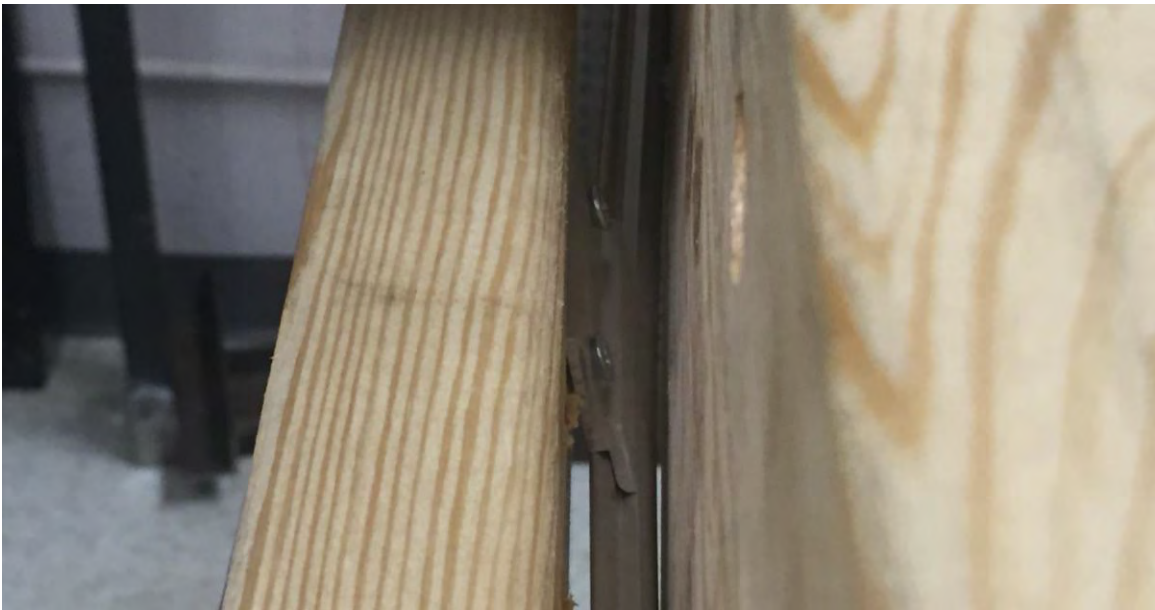
Figure 9. Bending of the 48" Z-Clip
