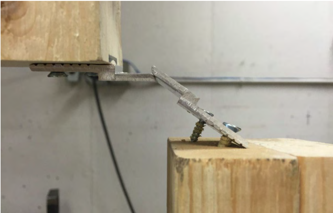
Figure 7. Screw Pullout Failure (Lateral Test)
