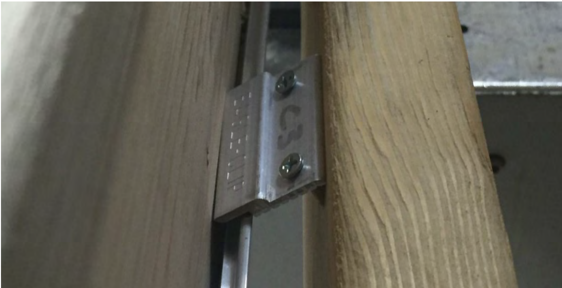
Figure 11. Screw Pullout of 2" Z-Clip opposite 48" Z-Clip.
