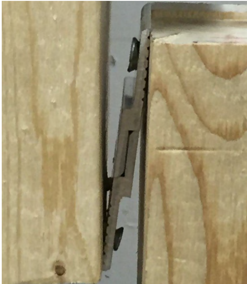
Figure 3. Vertical Load Test Screw Pullout
