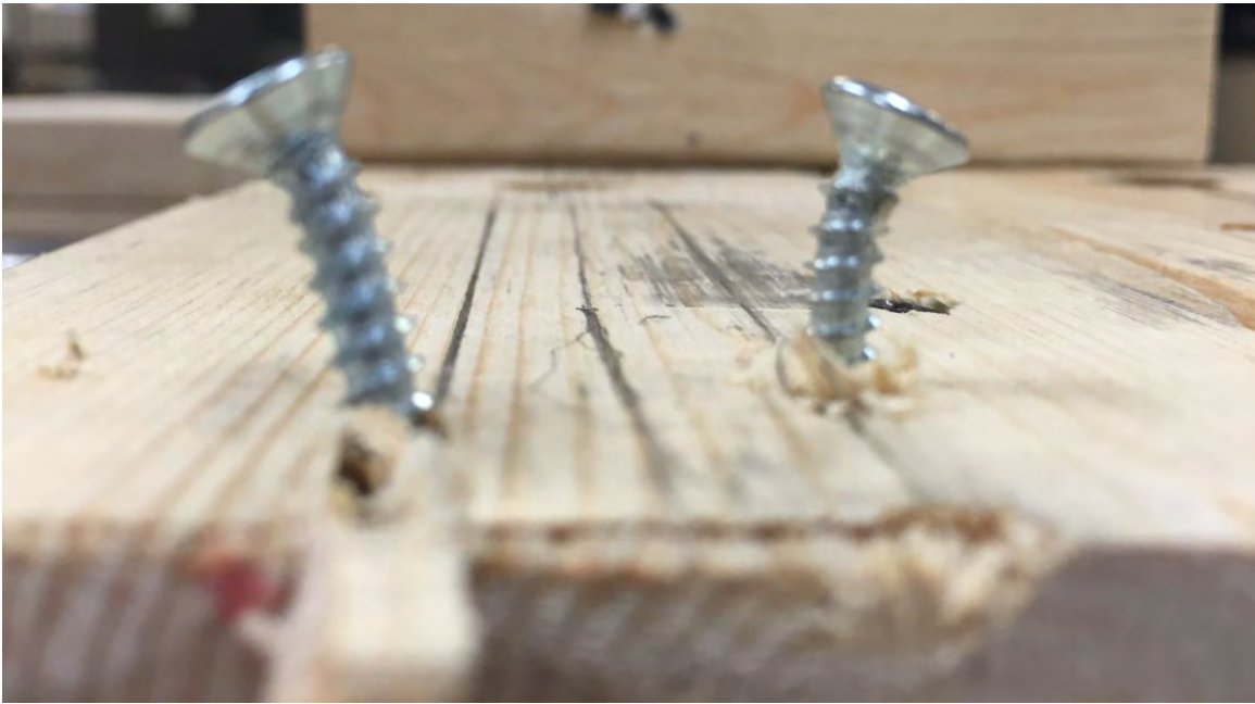
Figure 6. Wood Shearing Failure (Vertical Test)
