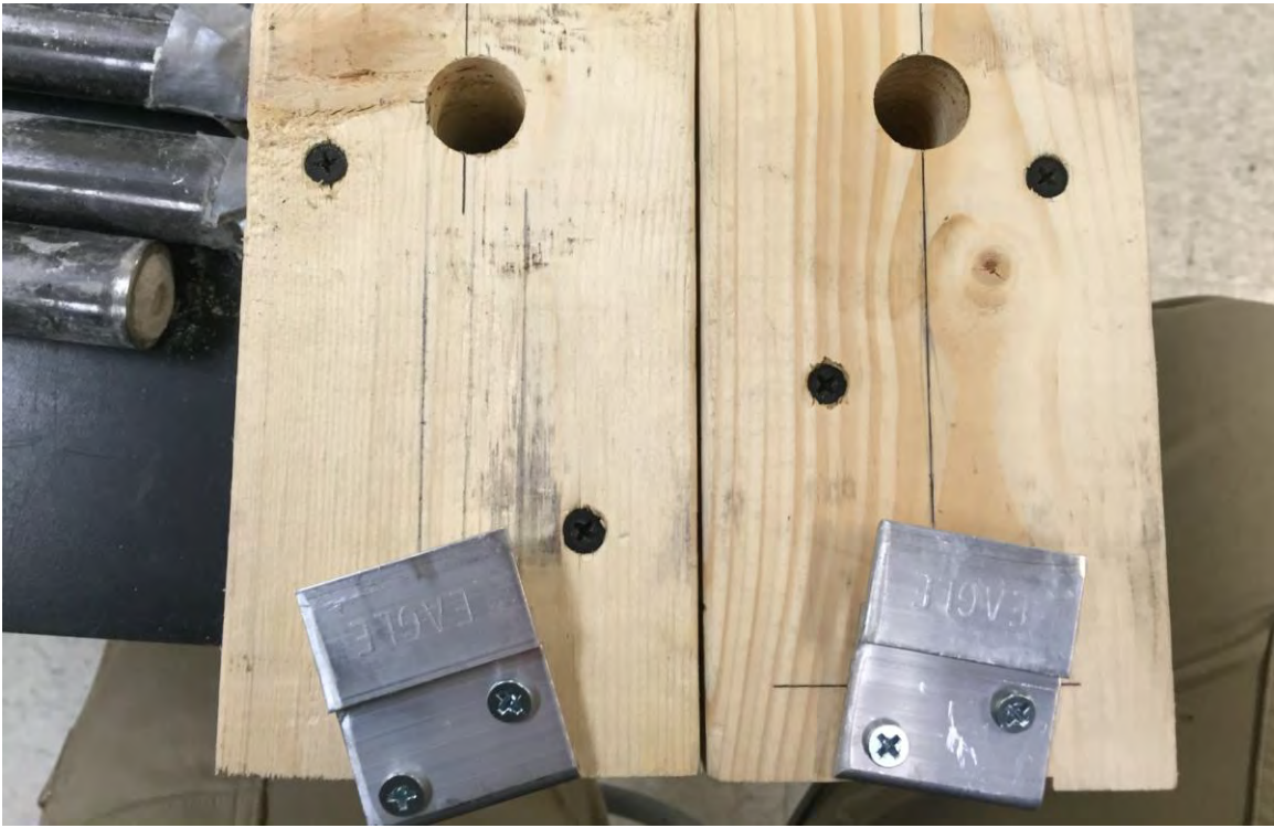
Figure 4. Wood Shearing Failure (Vertical Test)
