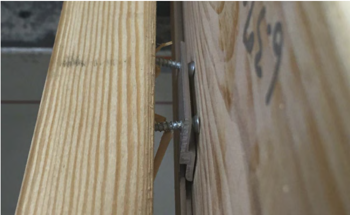
Figure 8. Screw Pullout of 2" Z-Clip opposite 48" Z-Clip
