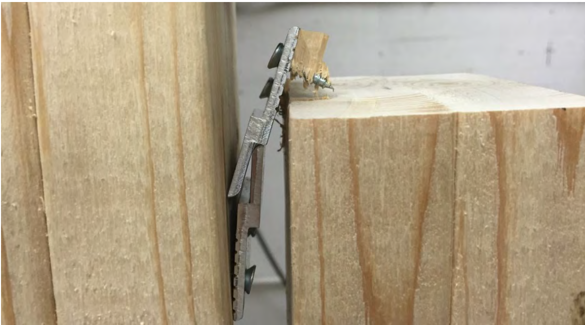
Figure 5. Wood Shearing Failure (Vertical Test)
