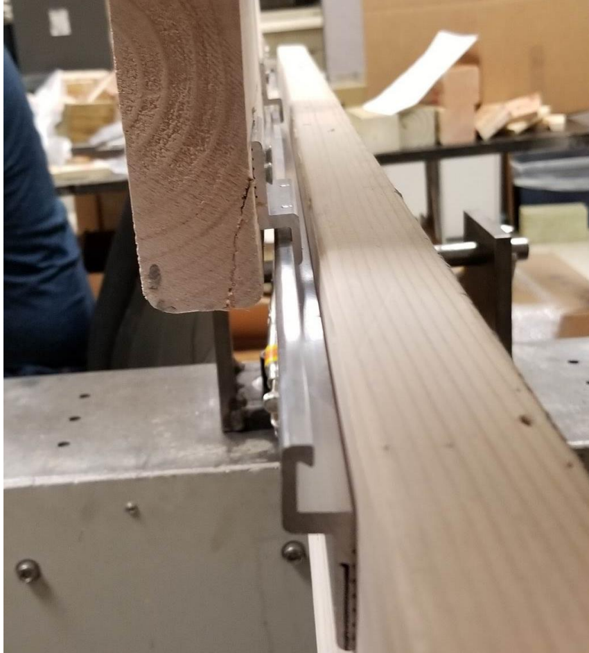
Figure 3. Clip Engagement (typical)
