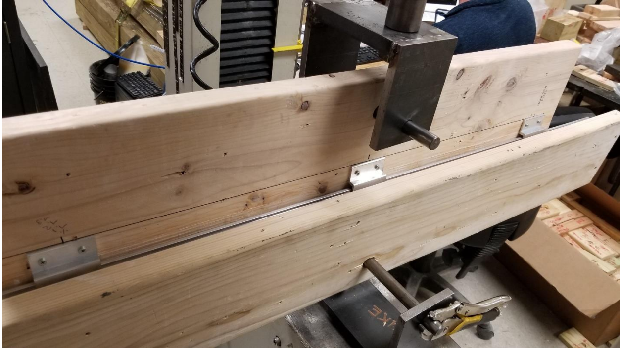
Figure 1. Vertical Load Test Setup (typical)
